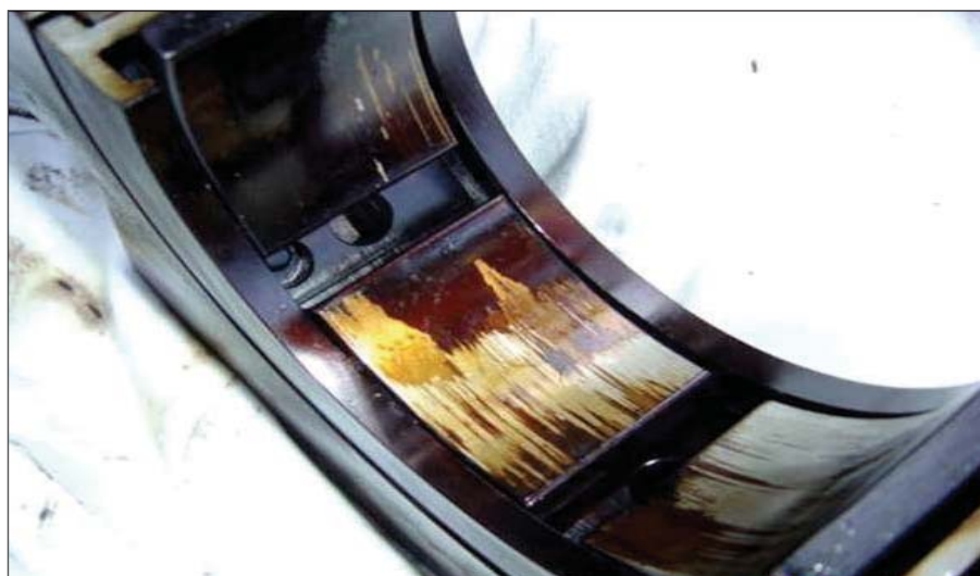
Figure 2 | Deposits on tilt bearing pads in a steam turbine.
