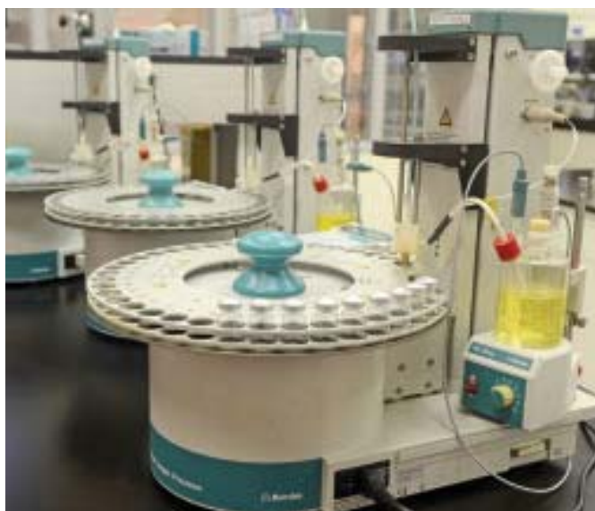
The Karl Fischer test measures the amount of water contained in a sample. A portion of the sample is measured and introduced into the Karl Fischer titrator. Any water present in the sample will react with the Karl Fischer reagents. The amount of reagent needed to react with the water present is measured and used to calculate the amount of water present. Results are given in parts per million (ppm) or percent.
