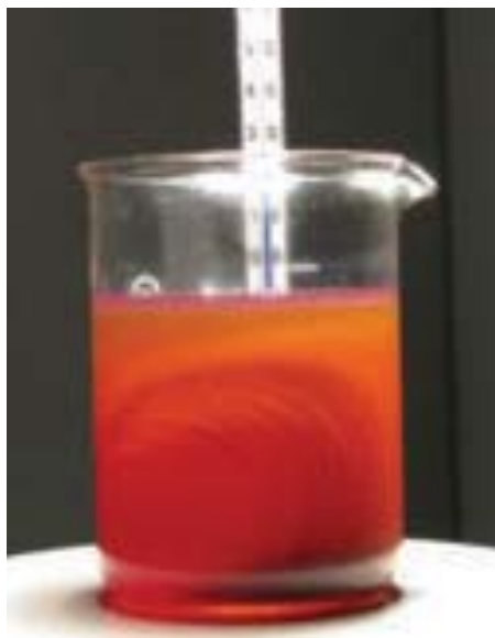
Figure 3 | At room temperature, this degraded oil is cloudy due to a high amount of soft contaminants. (Courtesy of Ansaldo Thomassen, The Netherlands)
