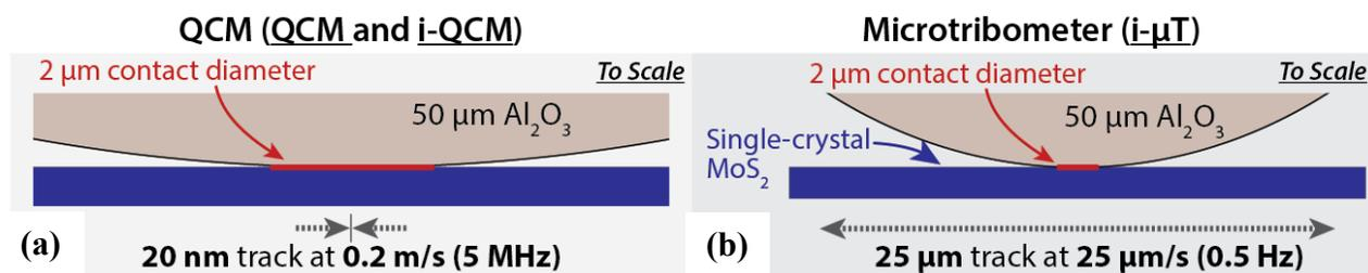
**Figure 1.** Schematic comparison of test conditions for alumina microspheres on substrates prepared with single-crystal MoS<sub>2</sub>. (a) The QCM reciprocates laterally at  $\sim 5$  MHz with a track length up to 50 nm and sliding velocity up to 0.5 m/s. (b) The track length in the spring-based tribometer is 25  $\mu$ m, with sliding speeds 5 orders of magnitude smaller than the QCM.
