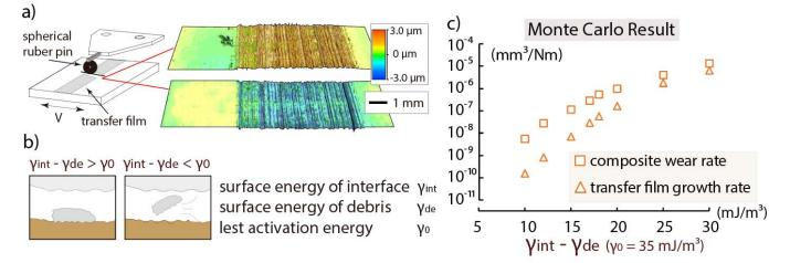
a) Removing pre-developed transfer films by sliding rubber ball; b) Relation between debris behavior and interface surface energy; c) Monte Carlo Result of interface fluctuation prediction model.
