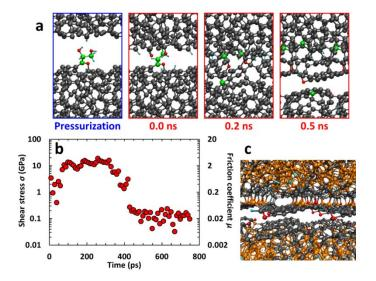
**Figure 1:** A QMD simulation of two ta-C surfaces lubricated with a glycerol molecule. (a) Snapshots of the 1-ns sliding simulation. (b) Evolution of the shear stress  $\sigma$  and friction coefficient  $\mu$ . (c) Shearinduced aromatic passivation of both ta-C surfaces. 3- and 4-fold coordinated C atoms are represented in grey and orange spheres, respectively.
