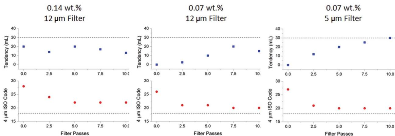
**Figure 3.** Foam tendency (top, squares) and 4  $\mu\text{m}$  ISO Codes (bottom, circles) for the 0.14 and 0.07 wt% treat rate additives filtered through 12- and 5- $\mu\text{m}$  filters. The dashed line indicates the maximum limits selected for this study and the color of the symbols indicates whether the spec was met (blue) or not (red). The results show that none of the cases tested here meet both particle count and foam targets.
