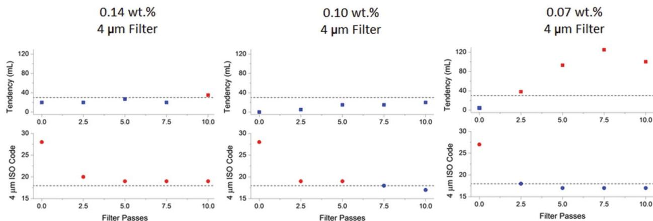
**Figure 4.** Foam tendency (top, squares) and 4  $\mu\text{m}$  ISO Codes (bottom, circles) for different treat rate additives filtered through the 4- $\mu\text{m}$  filter. Colors and dashed lines have the same meaning as in Fig. 3. With the 0.10 wt% treat rate (center) we observe that both particle count and foam targets are met after  $\sim$ 5–10 passes through the filter.
