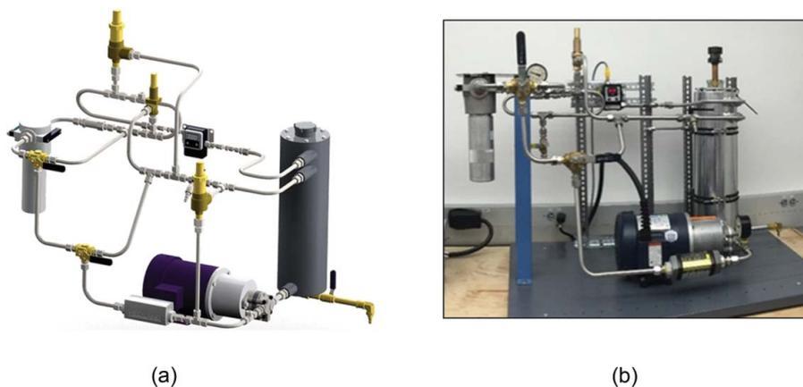
Figure 1. (a) Schematic and (b) photo of the custom-built filtration test rig that enables circulation, filtration, and particle counting of fluid samples.
