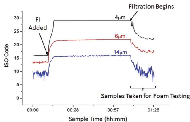
**Figure 2.** Representative particle count ISO Codes from the filtration test rig versus time. The increase in particle counts occurs when the FI is added to the system, and the particle count decreases after filtration.
