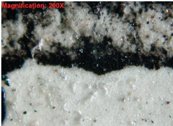
Figure 4 | A photomicrograph of precipitated additives that are produced due to contamination and removed by filtration is shown. (Courtesy of Filter Supplier No. 2)
