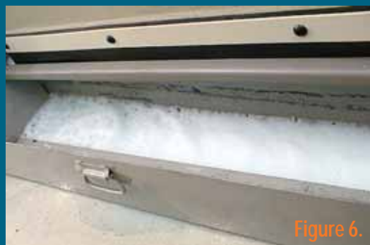
Figure 6. The higher speeds, flow rates, fluid velocity and pressure encountered with high-speed machining leads to a greater chance for the generation of foam.
