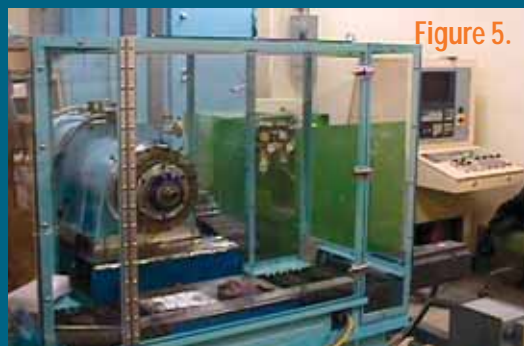
Figure 5. A machine tool with a 30,000 rpm spindle is used to study high-speed machining, model high-speed spindles and analyze chatter.
