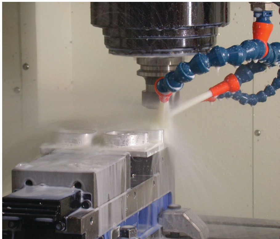
Figure 1 | Cutting fluid sprayed on a milling machine. (Photo courtesy of Glenn McKechnie.)
