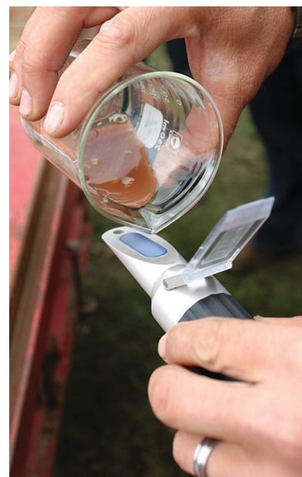
Figure 3 | Person pouring a fruit juice sample onto a refractometer plate.
