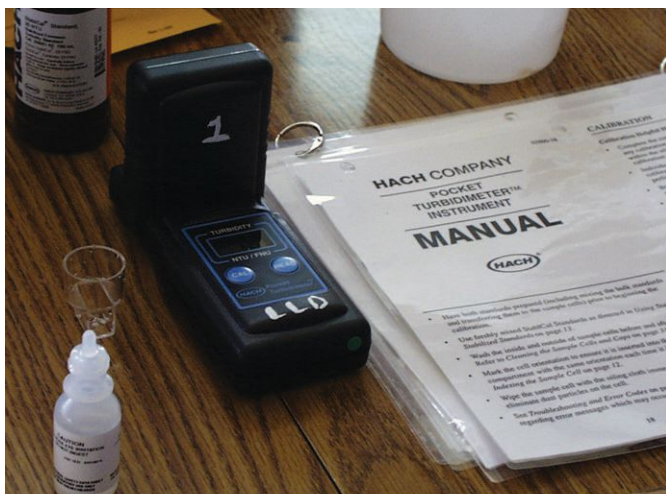
Figure 4 | A turbidimeter that tracks changes in fluid clarity. (Photo courtesy of www.lodi.gov/Storm_Drain_Detectives .)
