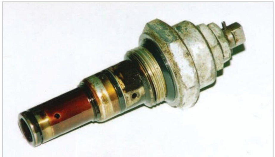
Figure 1 | A small layer of varnish deposit due to hydraulic oil oxidation can lead to servo-valve sticking, accelerated wear and malfunction. (Photo courtesy of A. Sasaki.)
