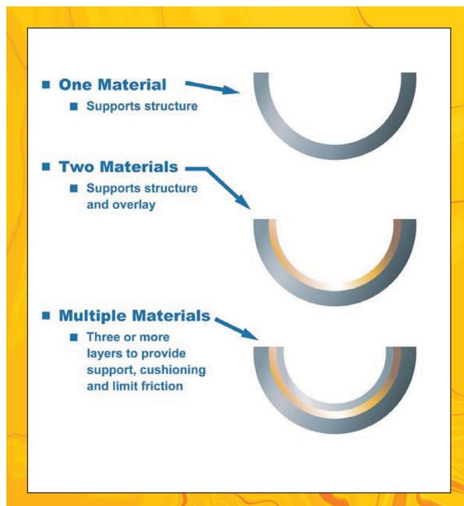
Figure 2 | Journal bearing construction (Courtesy of Trico Corp.)
