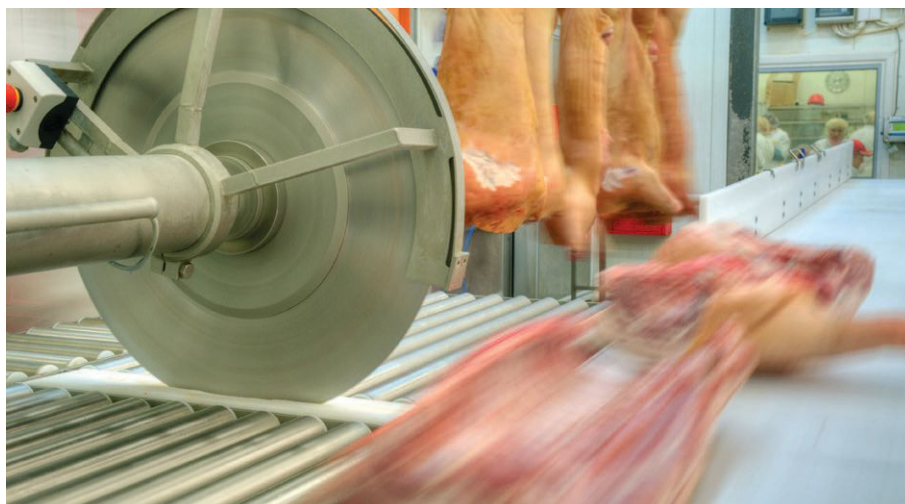
Food-grade machinery requires periodic lubrication; you can’t just slather any old type of grease on moving parts.
