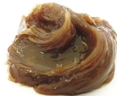
Figure 3 | Simple CS grease and simple Grade 2 CS grease have a more translucent appearance.
