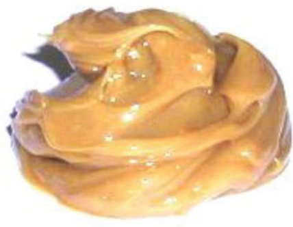
Figure 4 | Complex CS grease has an opaque appearance.
