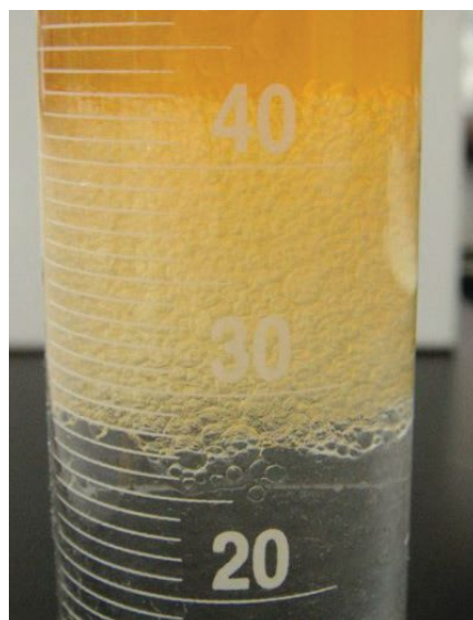
Figure 1 | Water separability test where oil is mixed with water in a heated bath.
