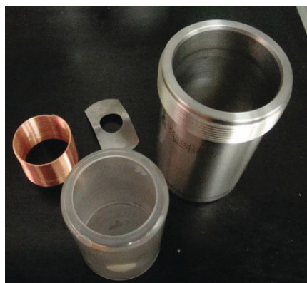
Figure 4 | The oxidative stability test where a portion of the oil is placed in a pressure vessel with water and a copper catalyst.
