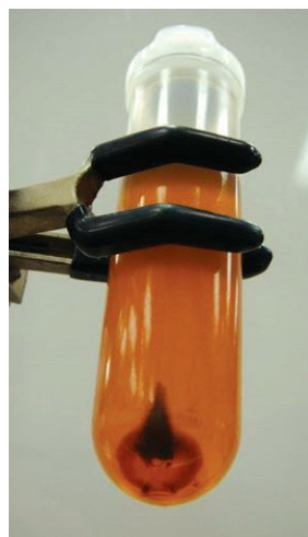
Figure 7 | The ultracentrifuge test. A portion of the oil is spun at a high speed in an ultracentrifuge, which causes higher density molecules to be forced to the bottom of the tube.
