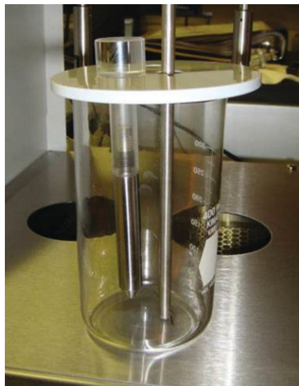
Figure 3 | The rust prevention test where a portion of the oil is placed into a vessel.
