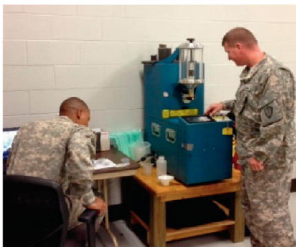
Soldiers perform on-site filter debris analysis (Courtesy of GasTops Inc.)
