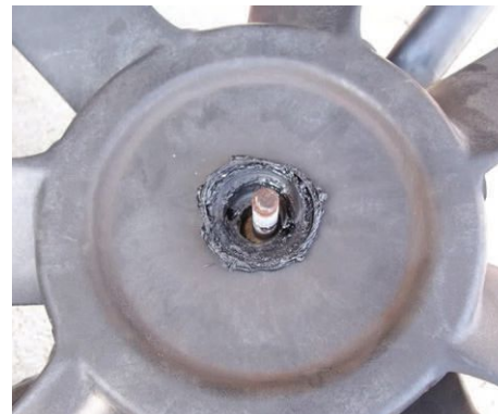
Figure 4 | Fan bushing thermal failure.
