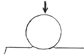
True Brinelling of Tapered Roller Bearing
