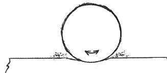
False Brinelling of Lubricated Tapered Roller Bearing
