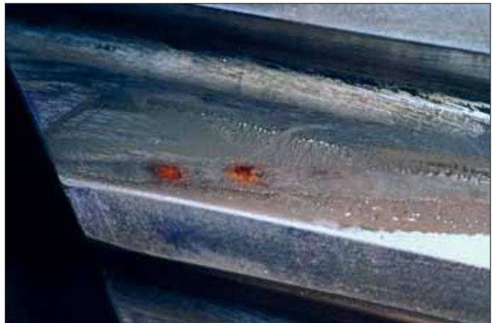
False brinelling on planet gear teeth.
