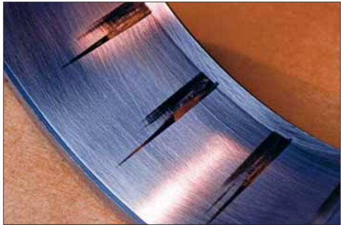
False brinelling and fretting corrosion in the outer raceway of a rolling-element bearing.
