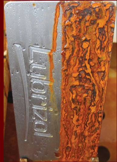
Figure 9 | Results on the salt spray test after 96 hours show that corrosion has just started on the side coated with the high-performance corrosion preventive.
