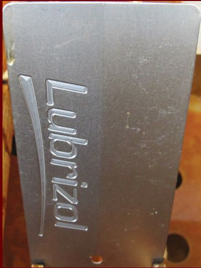
Figure 7 | Salt spray testing where the metal panel is coated with a high-performance corrosion preventive on one side and unprotected on the other side is shown at the beginning of the test.
