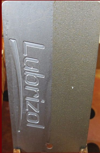
Figure 8 | Results on the salt spray test after 30 minutes show corrosion on the unprotected side.
