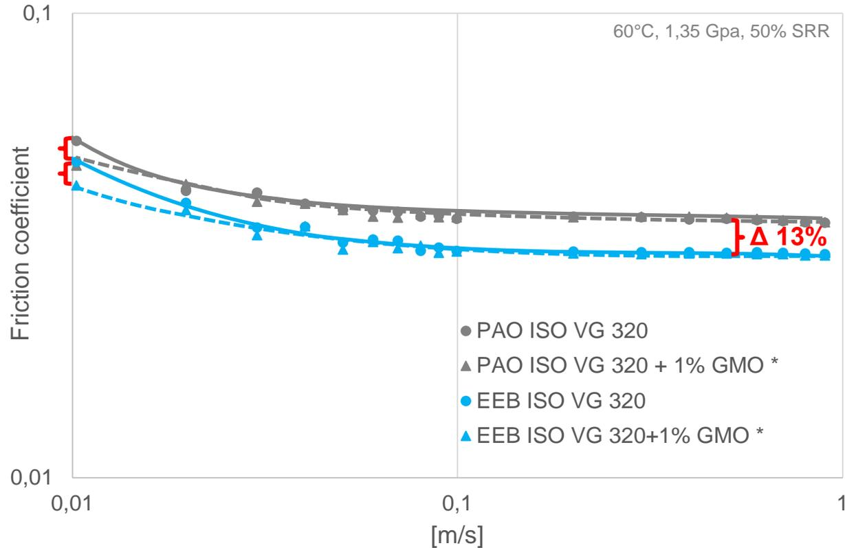
→ EEB reduces the friction coefficient in all friction regimes
