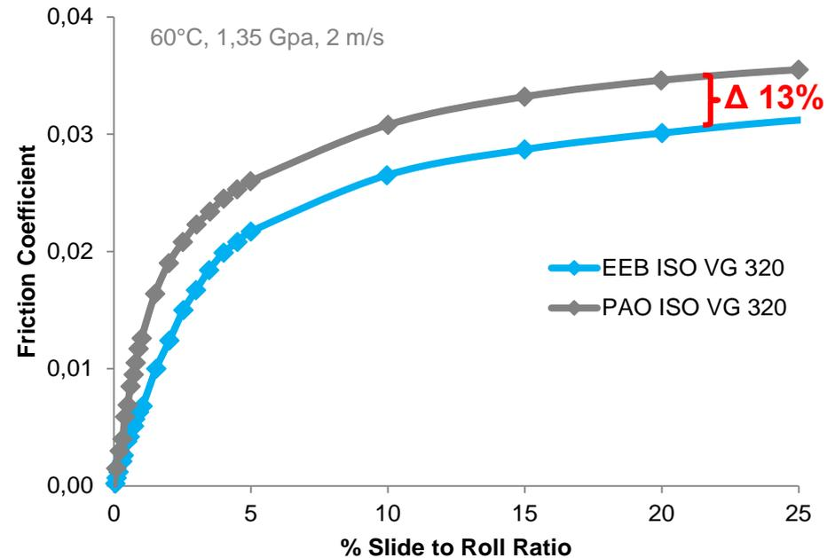
→ EEB based formulation reduces friction in fully formulated lube
