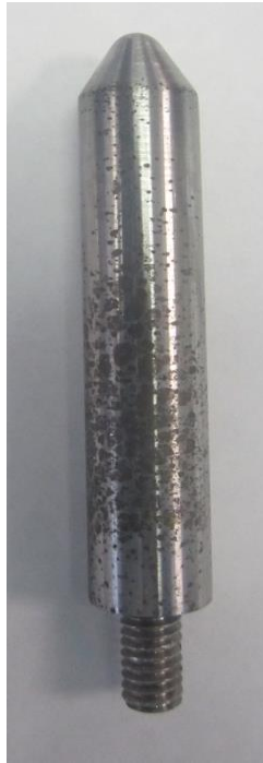
Sulfonate / Phenate 0.1% Fail
