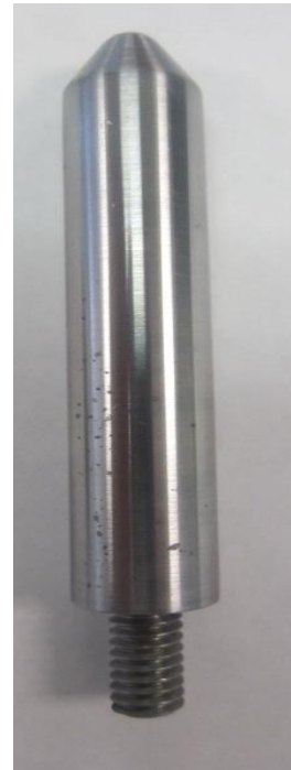
Sulfonate / Phenate 1.0% Fail
