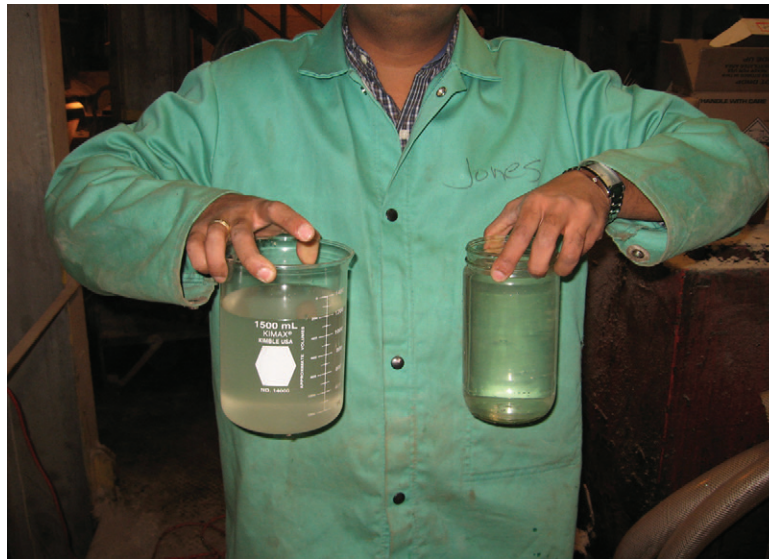
Figure 3 | The polymeric material known as the Hydrocarbon Removal Matrix can efficiently remove oil from wastewater effluent streams with droplet sizes between 0.1 micron and 15 microns. The beaker on the left shows the effluent from a glass plant prior to treatment. The clearer effluent after one pass through is seen in the jar on the right. (Courtesy of MyCelx® Technologies Corp.)
