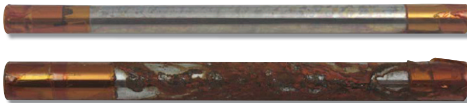
Figure 2 | After 1,100 hours of salt spray testing, a steel specimen coated with the nickel-tungsten alloy displays no rust in the top figure. In contrast, the same steel specimen coated with hexavalent chromium shows extensive rust in the bottom figure after only 48 hours. (Courtesy of the Massachusetts Institute of Technology)
