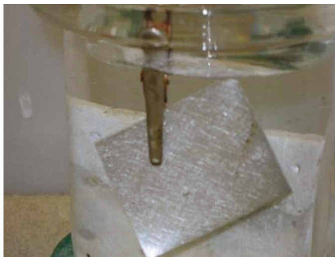
Figure 3 | The electrochemical process for using alane as a source of hydrogen can consume an aluminum electrode. The image on the left shows the aluminum electrode prior to the reaction of the alanate ion in THF. The image on the right shows the aluminum electrode consumed after the reaction. (Courtesy of the Savannah River National Laboratory)
