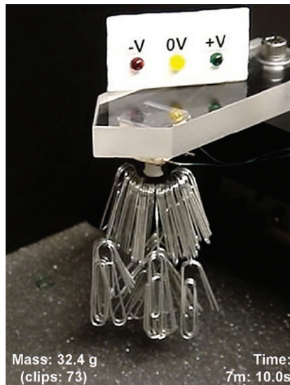
Figure 2 | Substrates can be reversibly attached to the SECAD, as shown with the placement of 73 paper clips weighing just over 32 grams in just over seven minutes. Adhesion is maintained until a release voltage is applied. (Courtesy of Cornell University)
