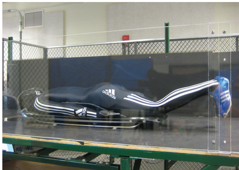
Figure 3 | A technique known as Digital Particle Image Velocimetry helps skeleton racers improve their ability to reduce aerodynamic drag. (Courtesy of Rensselaer Polytechnic Institute)
