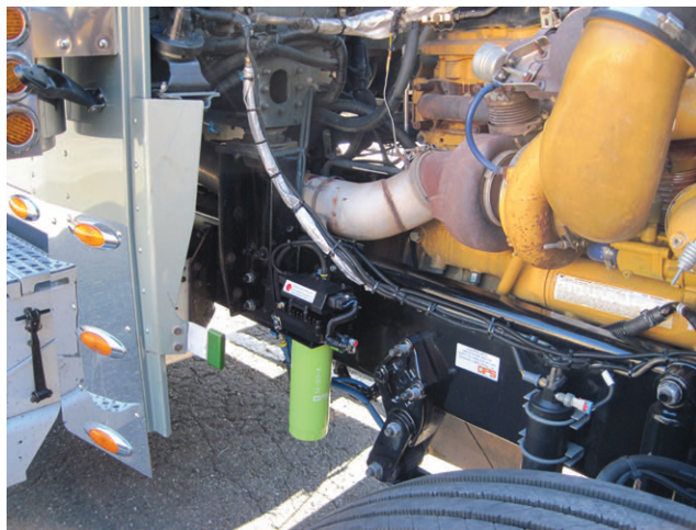
Figure 2 | A new technology installed onboard a vehicle has been developed that electronically monitors the condition of the lubricant and automatically adjusts processing to maximize contaminant removal. (Courtesy of Oil Purification Systems, Inc.)
